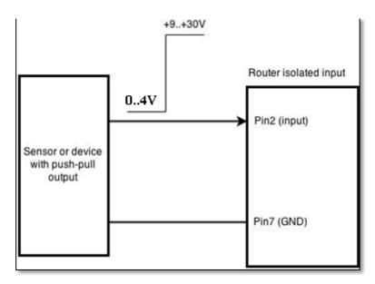
The signal source resistance should be less than 100 $\Omega$ .
