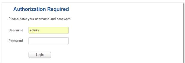
Enter the default password, which is "admin01" into the "Password" field and then either click Login with your mouse or press the Enter key. You have now successfully logged into the RUT955!
