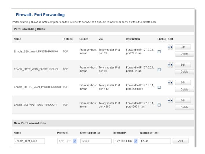
You can use port forwarding to set up servers and services on local LAN machines. The above picture shows how you can set up a rule that would allow a website that is being hosted on 192.168.1.109, to be reached from the outside by entering http://routersExternallp:12345/.
