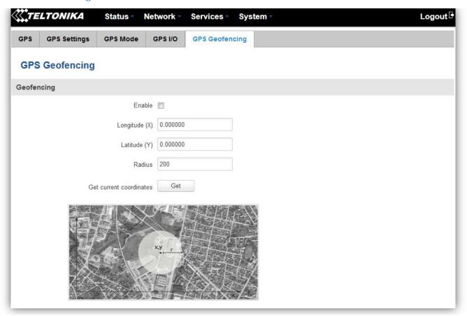
Geofencing is a feature which can detect whenever a device enters or leaves customized area.
