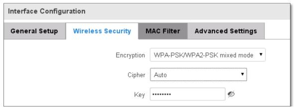
First select an encryption method: TKIP, CCMP, TKIP&CCMP and auto. Note: Some authentication methods won't support TKIP (and TKIP&CCMP) encryption. After you've selected your encryption method, you should enter your pass phrase, which must be at least 8 characters long.
