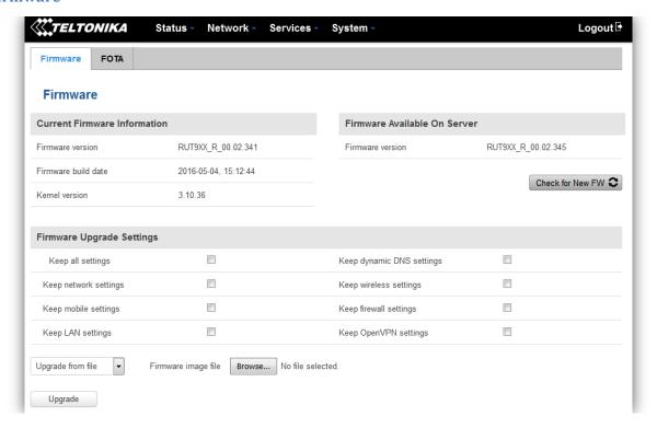
**Keep all settings** – if the check box is selected router will keep saved user configuration settings after firmware upgrade. When check box is not selected all router settings will be restored to factory defaults after firmware upgrade. When upgrading firmware, you can choose settings that you wish to keep after the upgrade. This function is useful when firmware is being upgraded via Internet (remotely) and you must not lose connection to the router afterwards.
