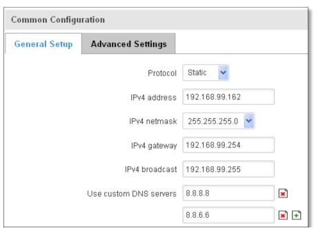
This is the configuration setup for when you select the static protocol.
