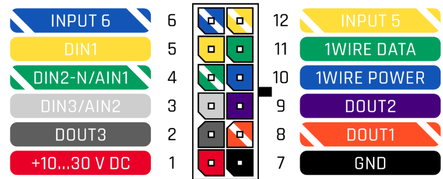
Figure 1 FMM230 2x6 socket pinout
