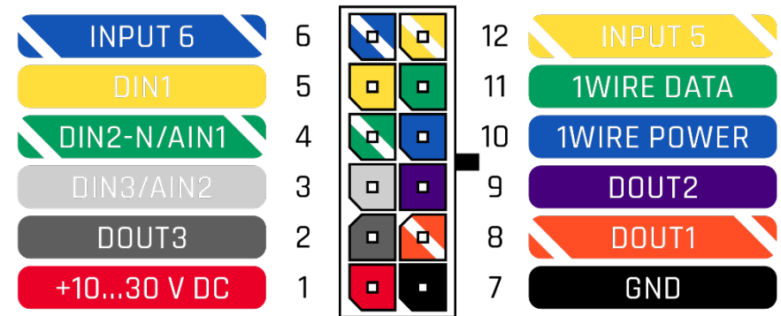
Figure 2 FMB230 2x6 socket pinout
