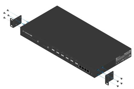
Attaching Rack-Mount Brackets to the EdgeSwitch Fiber
