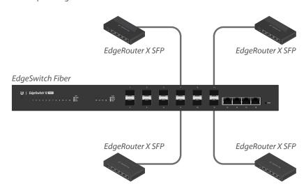
The EdgeSwitch Fiber connects multiple Ubiquiti EdgeRouter X SFP devices.
