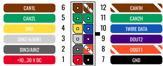
FMC150 2x6 socket pinout
